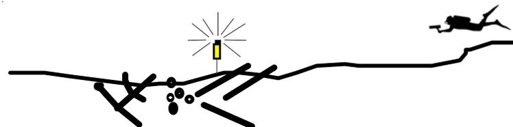
Pingers are available with different transmit frequencies so several can be deployed in the same general area without interference from each other. The diver adjusts his pinger receiver to the frequency of the desired pinger and the receiver leads him to it.
