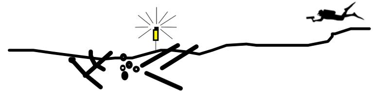
To mark an anchor line for returning divers, use the same setup as above and tie the pinger cord to the anchor line 6-10 foot up from the anchor (before deploying the anchor.)
